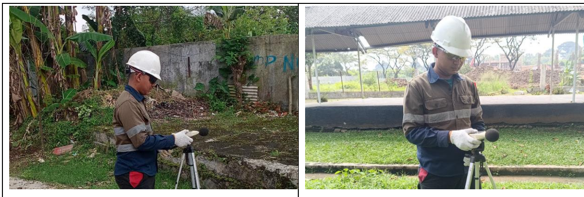
Figure 5.8 Noise Level Measurement
